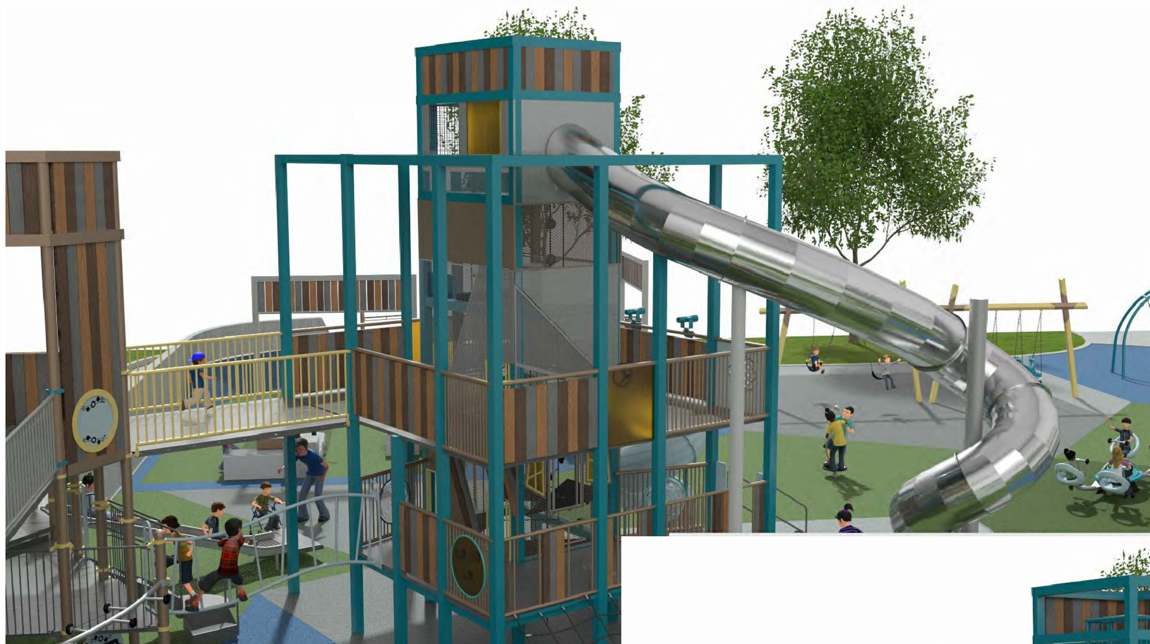
Above: Accessible Ramps Leading to Tower Feature with Railing and Panels Visible
