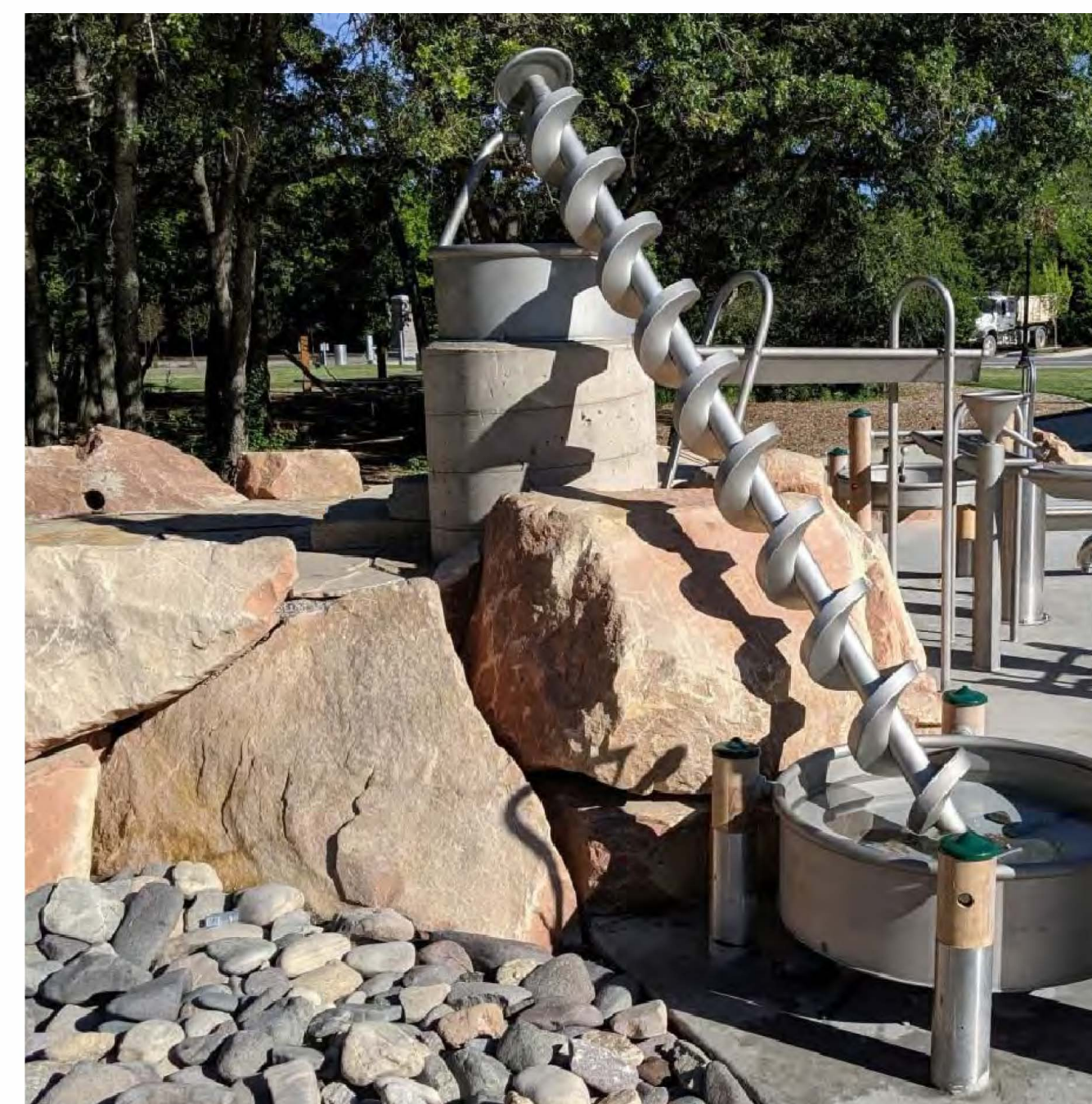
Above: Archimedes Spiral by Goric has an Accessible Hand Pump. The Spiral Pulls Water Up to The Upper Basin Where it Flows into the Raised Troughs.
