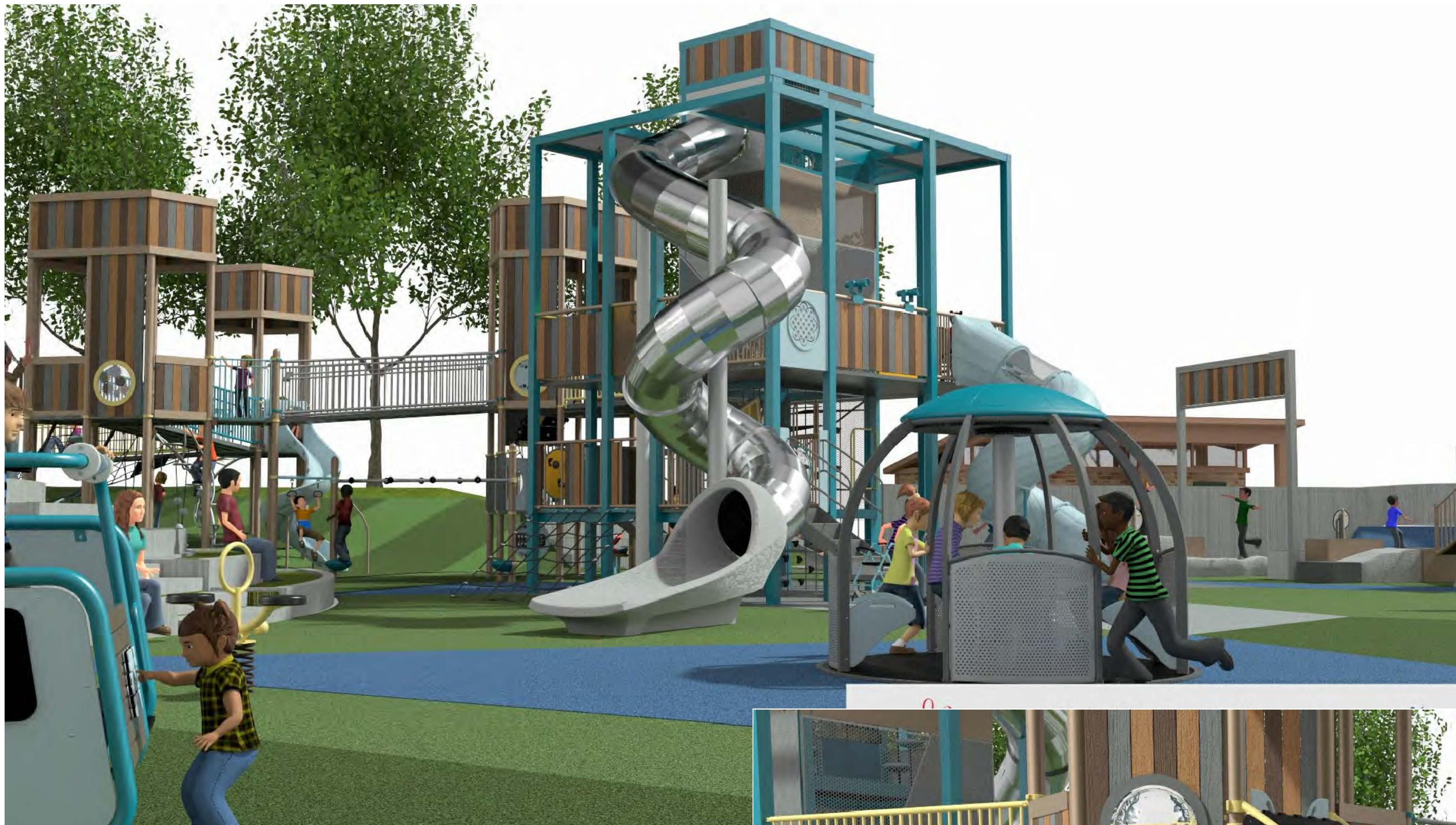
Above: Accessible Ramps Leading to Tower Feature. Features in the Foreground are 2-5 Play Structures with Some Accessible Features and Equipment. Background Right Shows the GFRC Rock Formations.
