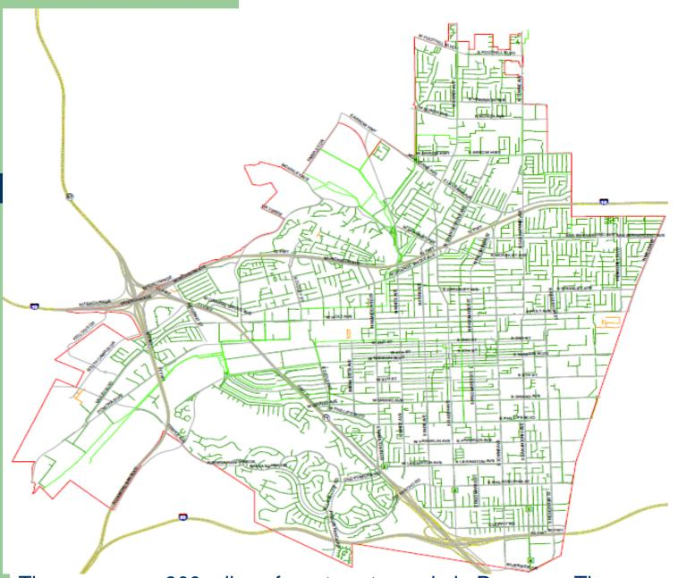
There are over 300 miles of wastewater main in Pomona. There are also over 30,000 service lateral connections to the wastewater mains.
